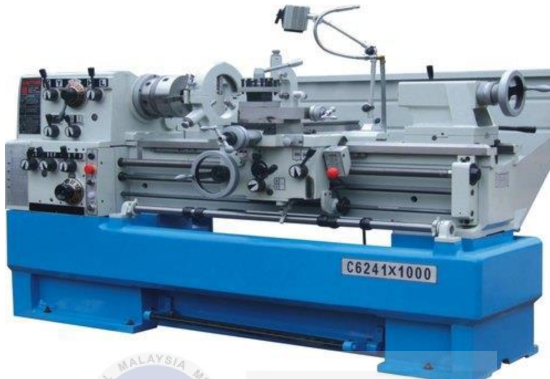
Figure 2.11 Example of engine lathe (Chauhan and Patel, 2020)
