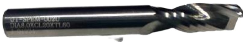
Figure 3.6: End mill carbide with diameter 8mm, 2 flutes and helix angle 30^\circ
