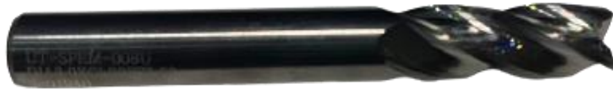
Figure 3.18: End mill carbide with diameter 8mm, 4 flutes and helix angle 30°
