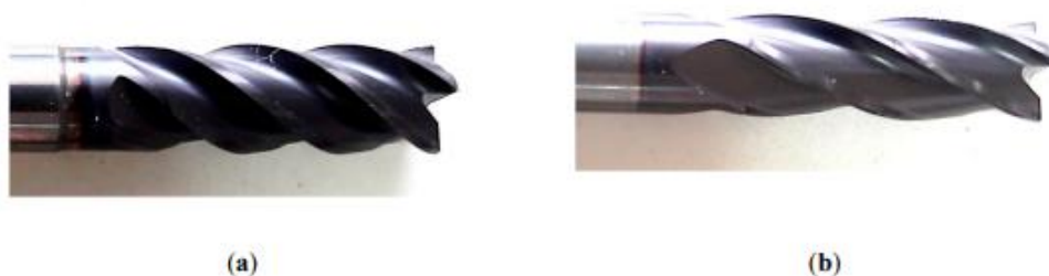
Figure 2.12: Ceramic-coated tungsten carbide side and end-mill cutters having helix angles of (a) 42° and (b) 30°.
