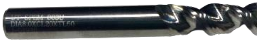
Figure 3.8: End mill carbide with diameter 8mm, 2 flutes and helix angle 50°
