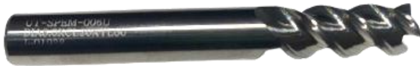
Figure 3.14: End mill carbide with diameter 8mm, 3 flutes and helix angle 50°
