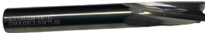
Figure 3.16: End mill carbide with diameter 8mm, 4 flutes and helix angle 10°
