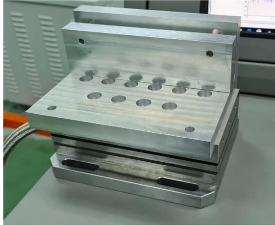
Figure 3.7: Jig to hold the specimens.
