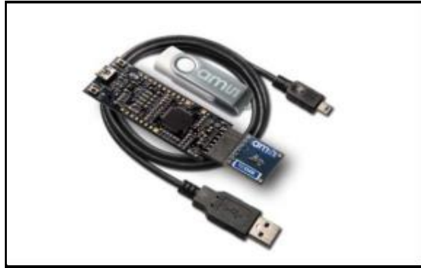
FIGURE 2-9 TCS3400 Colour Sensor [34]
