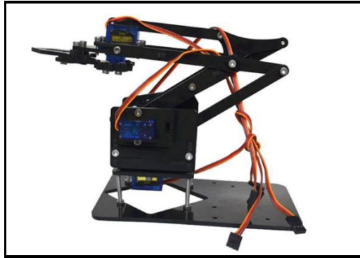
FIGURE 3-4 4DOF Robot Arm [69]
