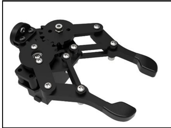
FIGURE 2-6 Example of claw gripper [25]
