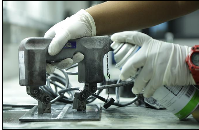
Figure 2.1 : Magnetic Particle Inspection
