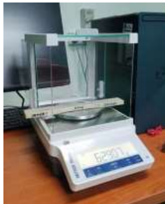
Figure 3.13 The sample are weighted by analytical balance.
