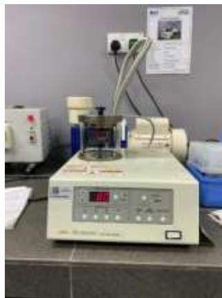
Figure 3.15 The sample in the sputter coater
