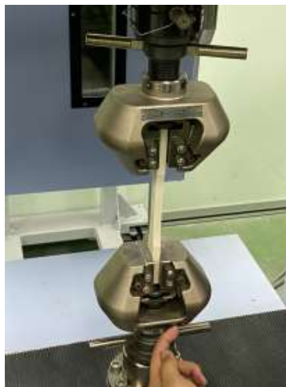
Figure 3.8 Specimen has been Setup Before the Tensile Test
