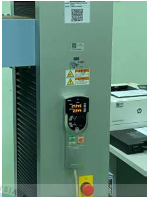
Figure 3.5 Smart Control Panel of the Shimadzu Universal Tensile Machine
