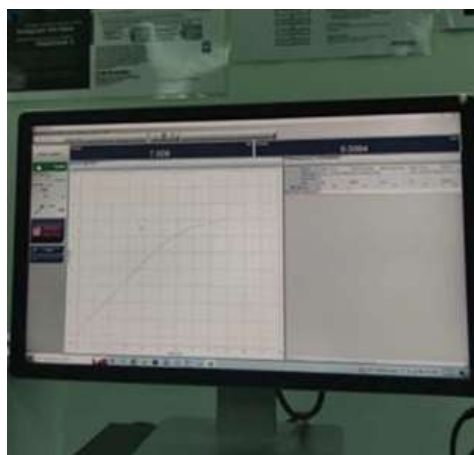
Figure 3.7 Trapezium-X Lite that connect with the Shimadzu Universal Tensile Machine
