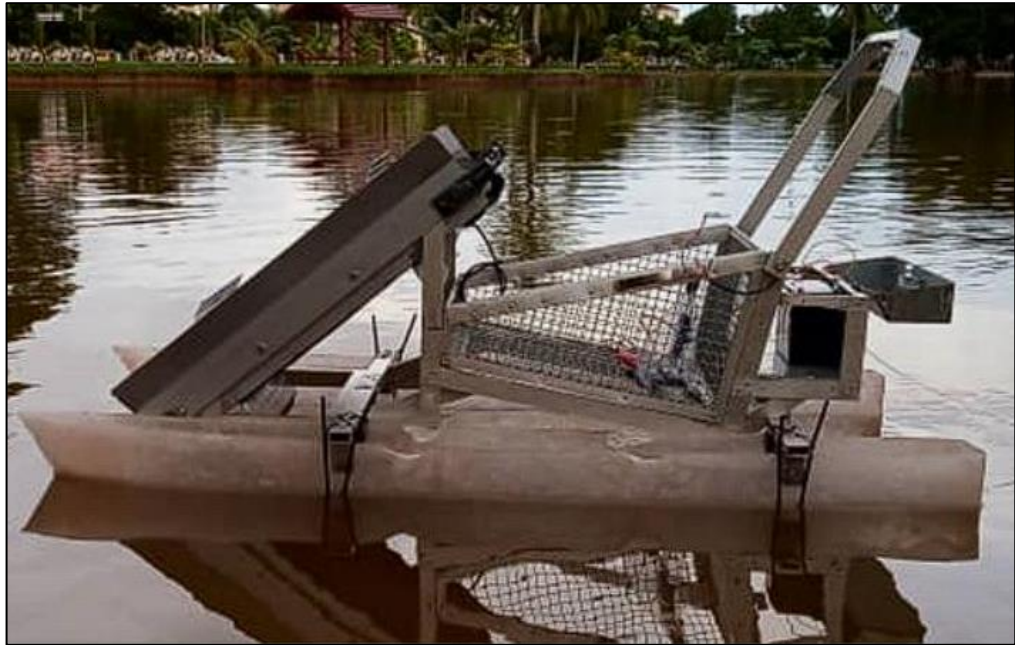
Figure 9 Miniature model of UniSZA's Portable Trash Collector Boat
