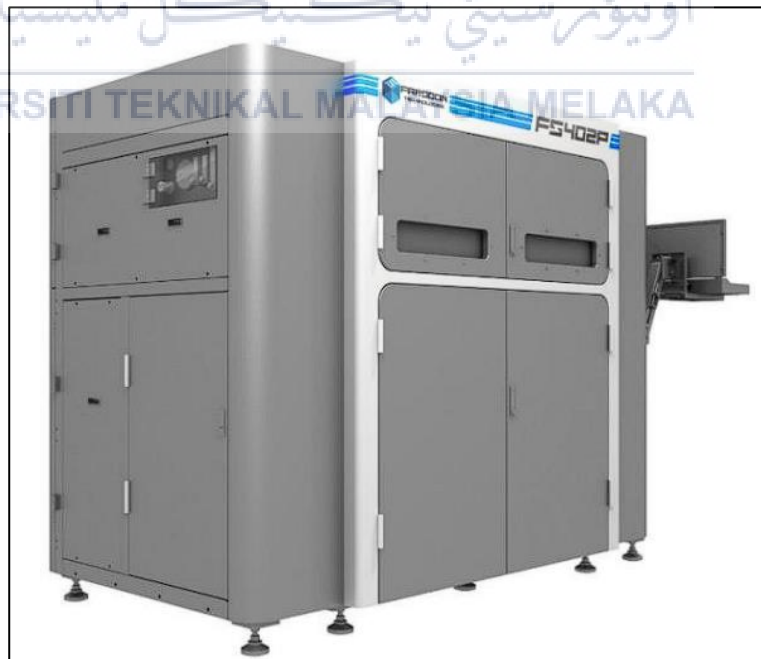
Figure 12 Farsoon SS402P Selective Laser Sintering (SLS) machine (Farsoon Technologies, 2017)
