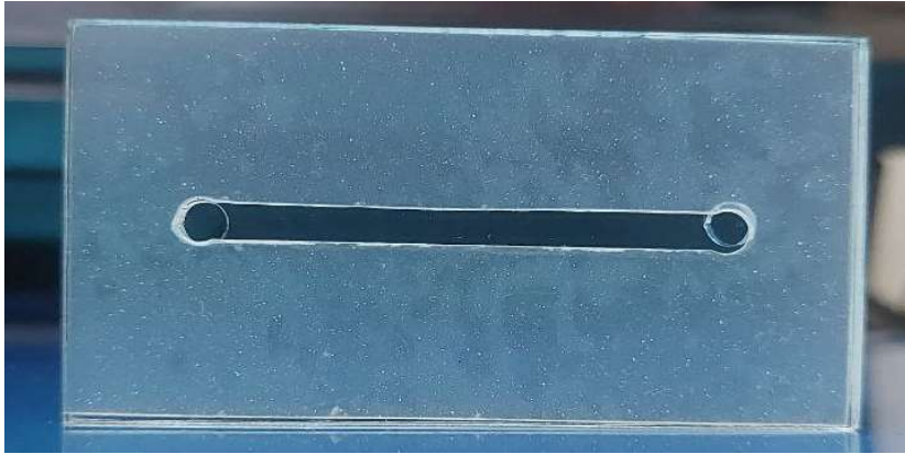
Figure 4.8 2.5mm Microchannel Biosensor Fabricated using Laser Engraving Method
