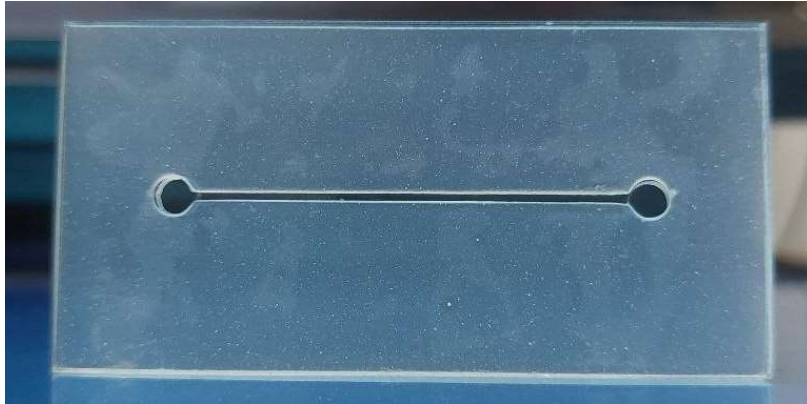
Figure 4.10 0.25mm Microchannel Biosensor Fabricated using Laser Engraving Method
