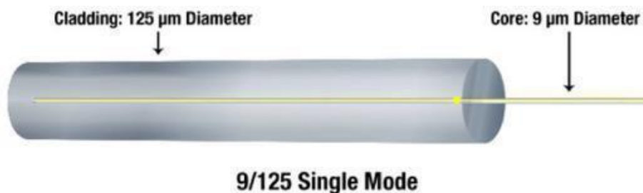
Figure 2.2 Single Mode for Light Path
