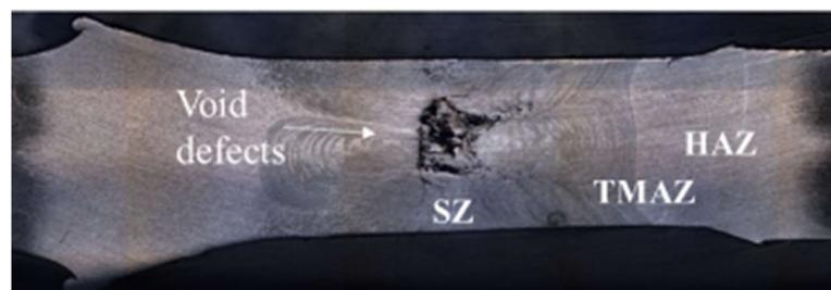
Figure 2.7 Void defect formed under 400rpm and tool traverse speed of 120 mm/min.
