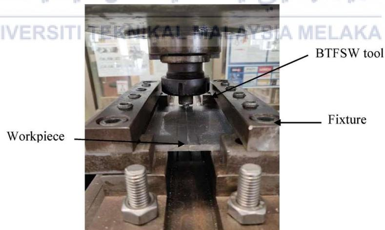
Figure 2.3 Configuration of Bobbin friction welding (Fuse & Badheka, 2020)
