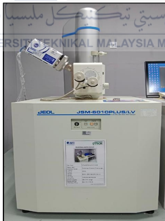
Figure 3.7: SEM-EDS machine (JEOL JSM-6010PLUS/LV) (Material Science laboratory)
