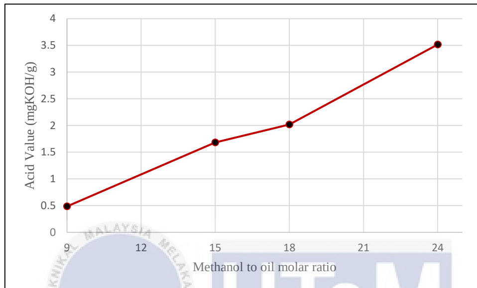
Figure 4.2: Graph for different methanol to oil molar ratio (9:1, 15:1, 18:1 and 24:1) with catalyst 9% versus acid value mgKOH/g
