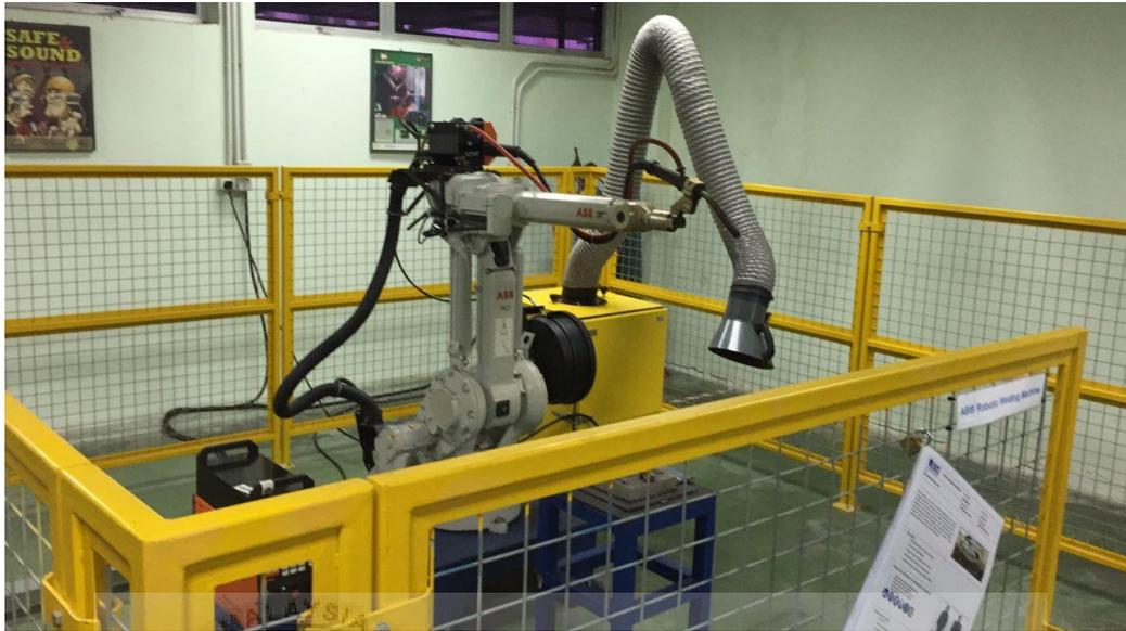
Figure 3.13: IRB 1410 M2004 robot welding
