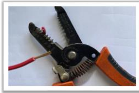
Figure 3.37: Wire stripper removing the wire insulation
