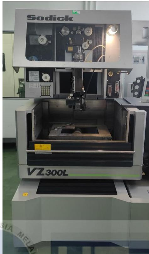
Figure 3.10 Sodick VZ300L EDM wire-cut machine.
