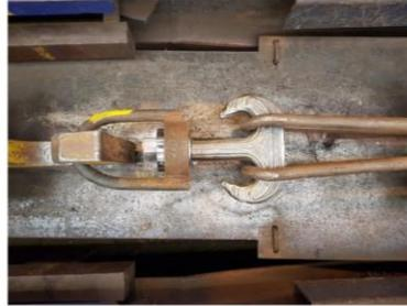
Figure 2.13D printed WAAM hook (Khodabakhshi & Gerlich, 2018)
