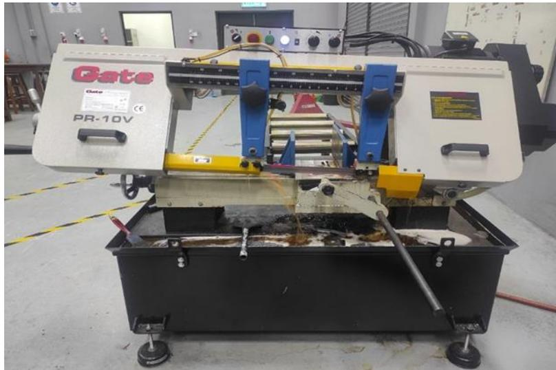
Figure 3.8 Horizontal Band sawing Machine PR-10V
