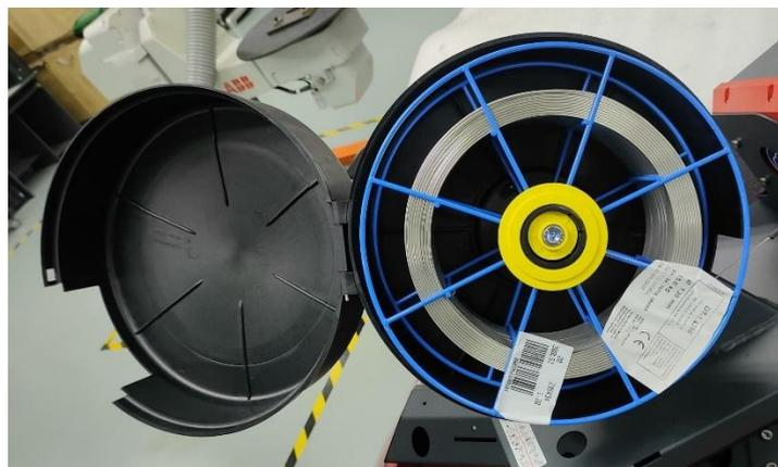
Figure 3.2SS308LSi Stainless Steel LSi
