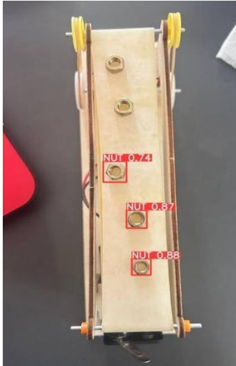
Figure 4.11 : Nut detection on conveyor belt
