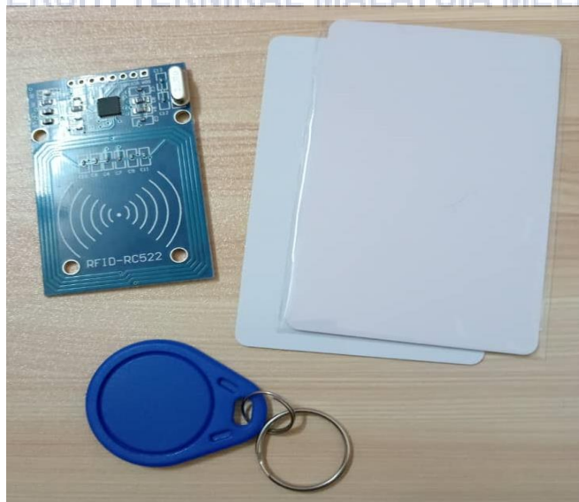
Figure 3.6 RFID cards, keychain and MFRC255 module
