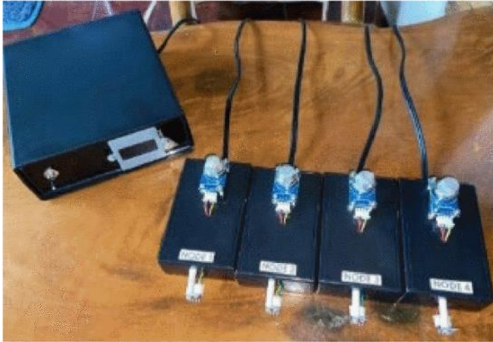
Figure 2.1.2 The PHOENIX: A wireless ESP32 mesh network for fire detection and monitoring system.[7]
