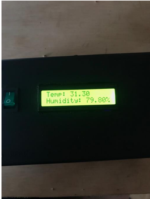
Figure 4.4 LCD show reading temperature, humidity and moisture.
