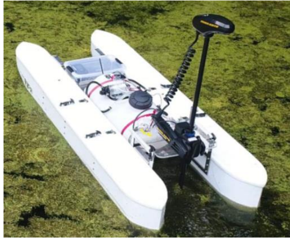
Figure 2.3 Autonomous Robotics for Identification and Management of Invasive Aquatic Plant Species [3].
