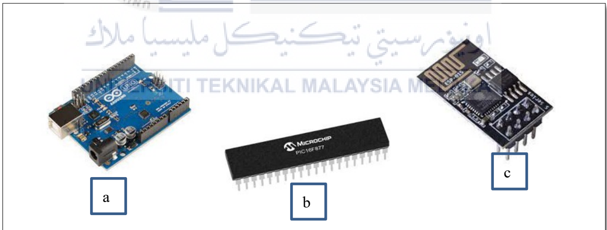
Figure 2.9 (a) Arduino Uno, (b) PIC 16F877, (c) ESP8266 Wi-Fi Module
