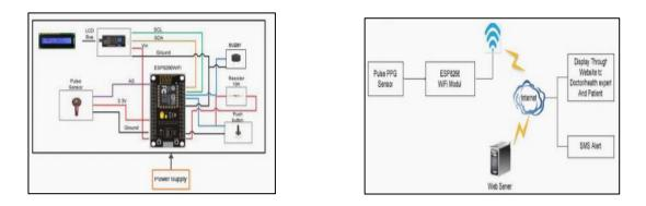
(a) Pulse sensor with ESP8266 module
