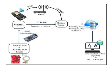
Proposed Architecture of IoT based ECG monitoring system.
