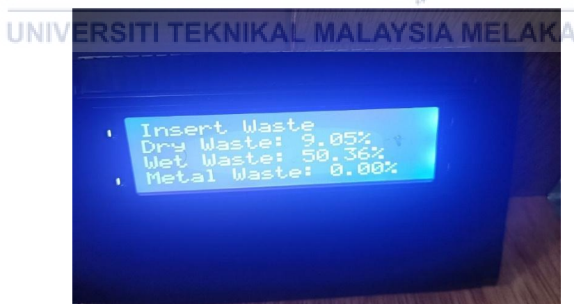
Figure 65: LCD display status of Bin level
