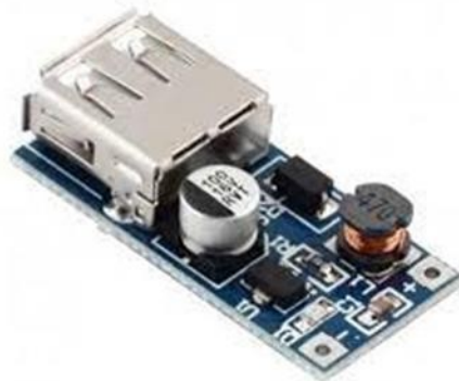
Figure 3.10 DC-DC Booster Module (0.9-5V)
