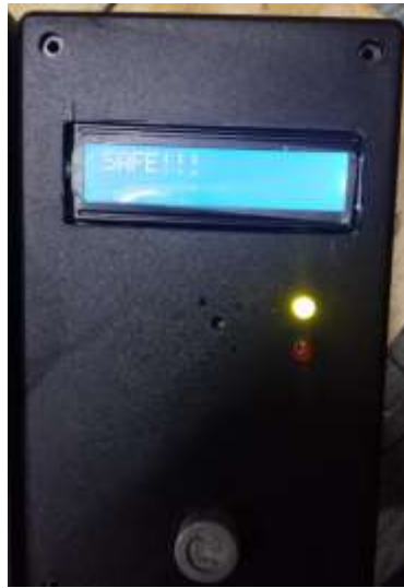
Figure 4. 4 Green LED turn on in normal condition
