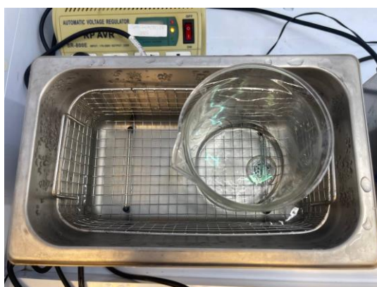
Figure 3.11 Sonication process to clean the glass substrate beakers.
