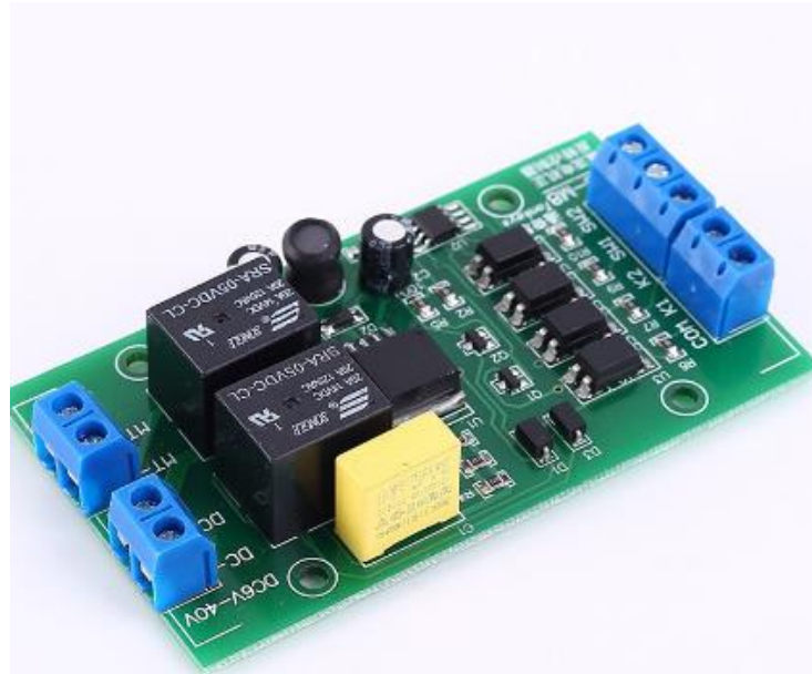
Figure 3.18 Design of the hardware DC Motor controller high current board.
