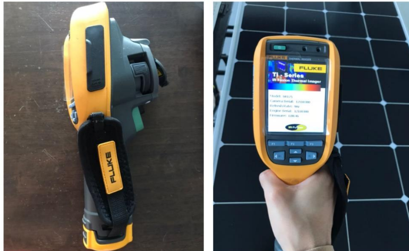
Figure 29 Infrared Thermal Imager
