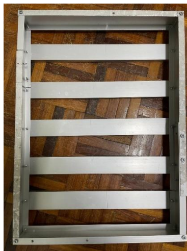
Figure 4.1 Frame Mounting Structure without Fins
