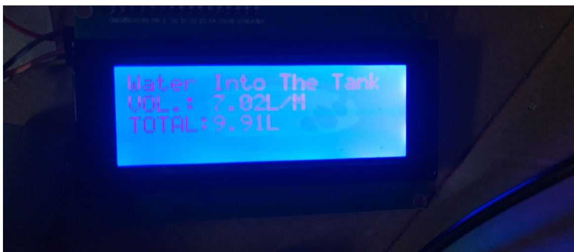
Figure 4.22 Flowrate and volume displayed on i2C LCD display
