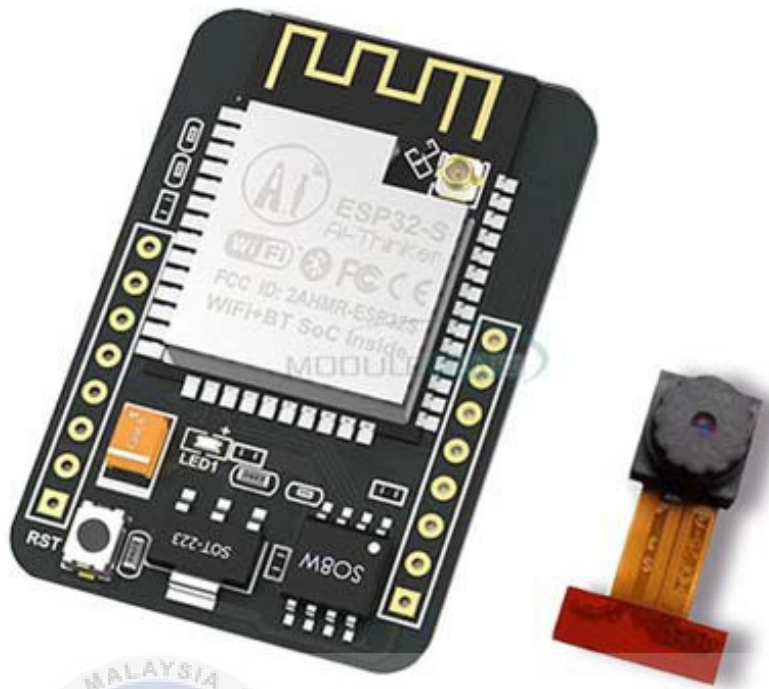
Figure 2.9 ESP32 with the camera module[44]
