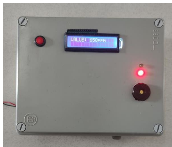
Figure 4.6 Red LED light on when value exceed 500ppm.
