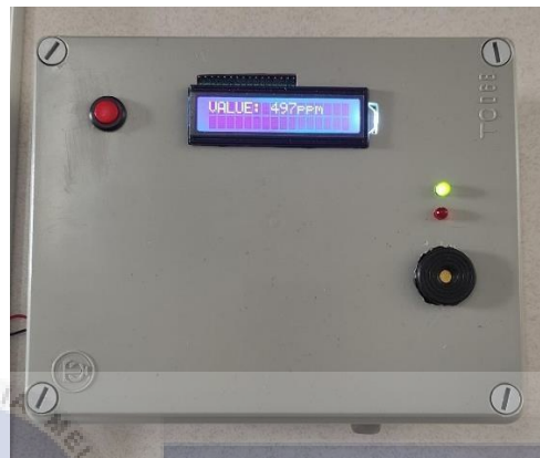
Figure 4.5 Green LED light on in normal condition.
