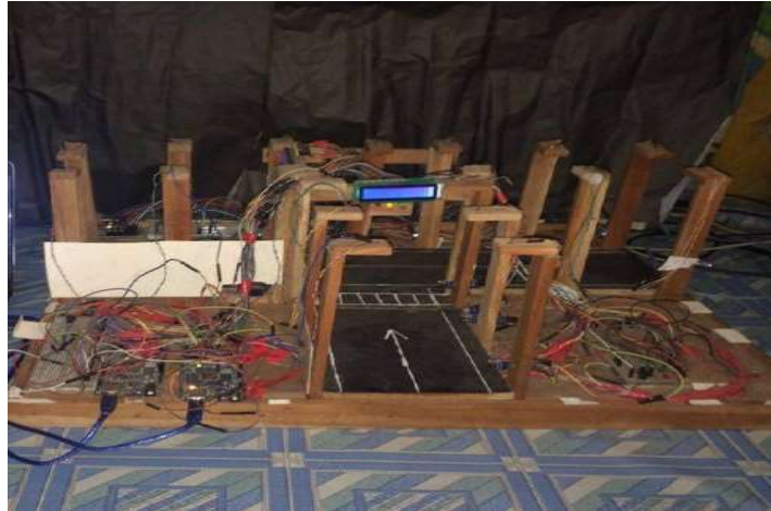
Figure 3.1 Prototype of the IoT based system for smart street light [13]
