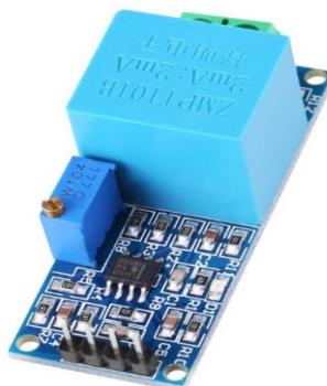
Figure 3.5 AC Voltage Sensor ZMPT101B [19]
