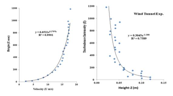
Figure 3.5 Wind tunnel experimental study velocity profile (U) and turbulence intensity (I) used for CFD simulation (Sanyal & Dalui, 2018)
