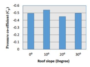
Figure 4.11 Maximum pressure coefficients (area weighted average) for different roof slopes
