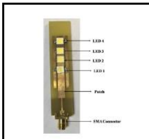
Figure 2. 16 The Product Structure Antenna with LED
