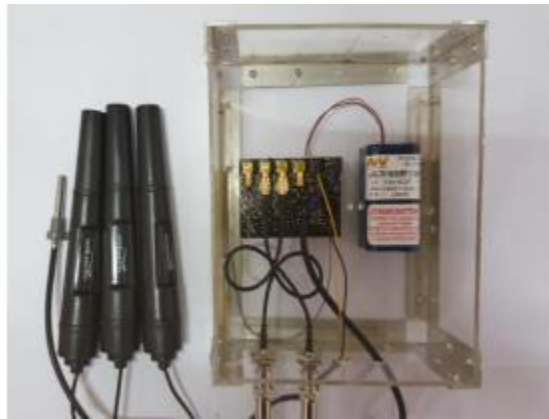
Figure 2-4 Deployment Setup with the sensors and Waspote microcontroller board [5]
