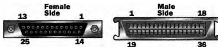
Figure 2-2: PC's parallel port for printing purpose
