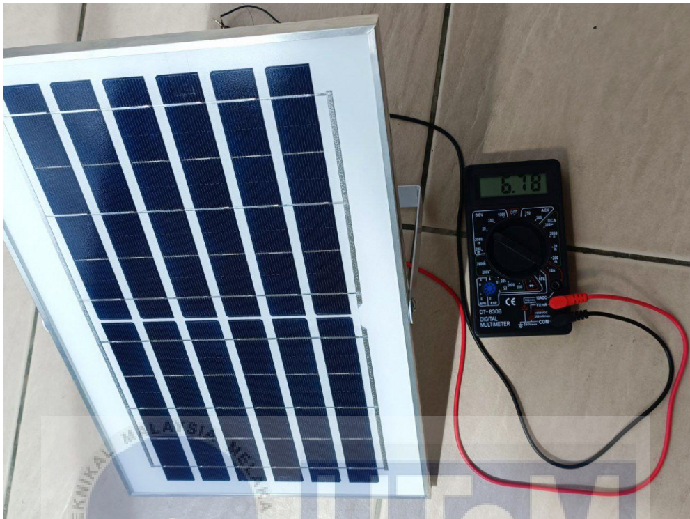
Figure 4.18 Measure the output voltage (V) and current (A) of the solar panel
