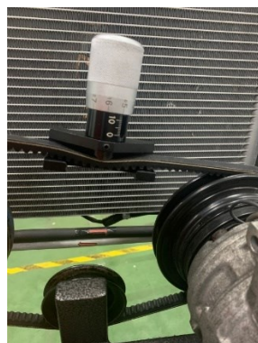
Figure 3.5 Tensioning Gauge to Measured Deflection Belting
