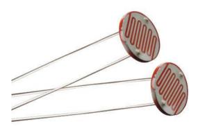
Figure 3.2; Light Dependent Resistor [29]
