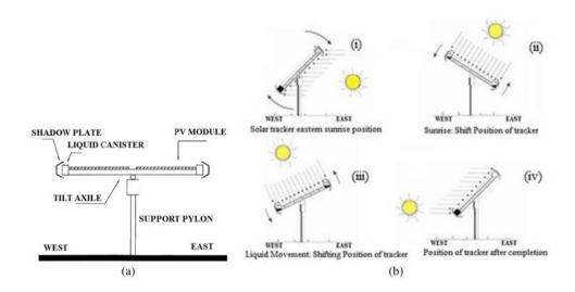
Figure 2.8; Shows how does a passive solar tracker works. [23]
