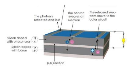
Figure 2.2; Ilustration on how a photovoltaic cell works.[11]
