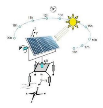
Figure 2.6; Shows how a chronological solar tracker works. [18]
