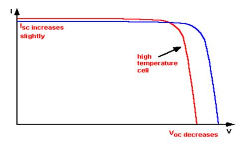
Figure 2.3; The effect of temperature on the IV characteristics of a solar cell.
