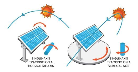
Figure 2.9; Single axis solar tracker [25]
