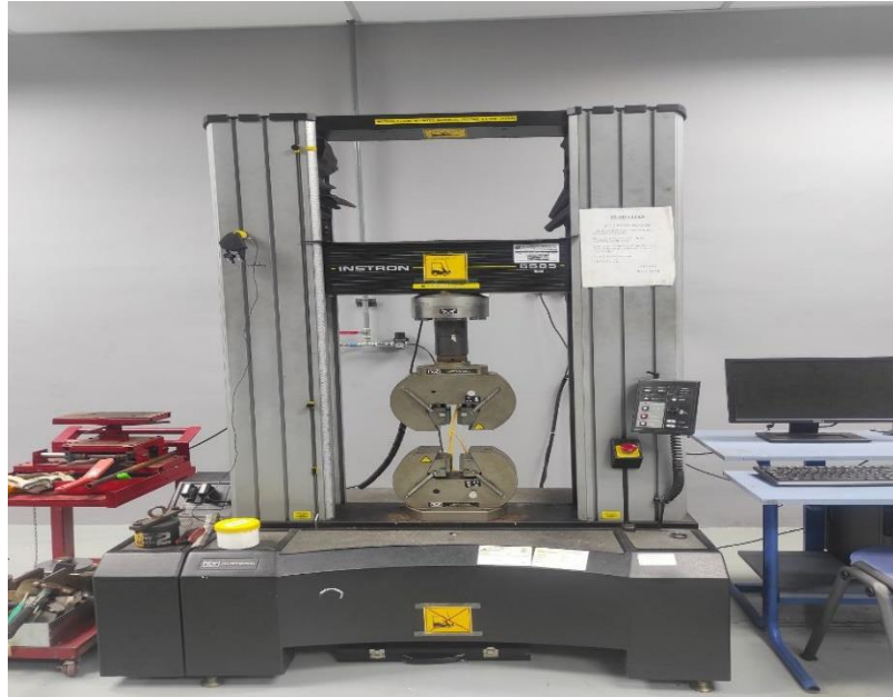
Figure 3.42 Floor-Mounted Material Testing System. Instron Model 5585 Capacity 200KN.
