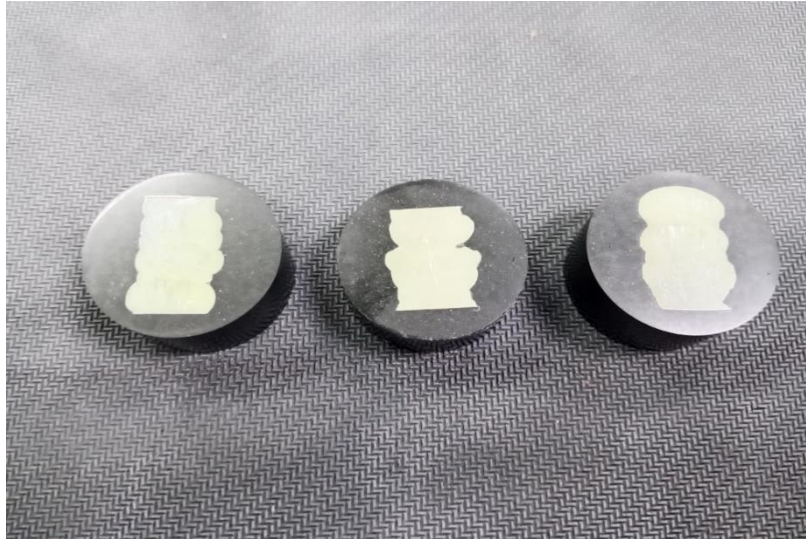
Figure 3.66 The specimens were encapsulated by using hot mounting presses. From left bottom, centre and top.
