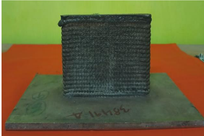
Figure 2.12 Fabricated SS316L wall. (Senthil et al., 2023)
