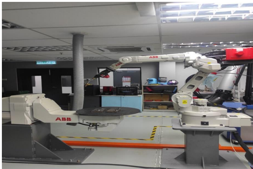
Figure 3.12 Robot arm and welding torch. IRB 2600ID
