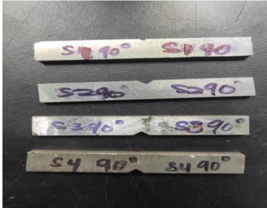
Figure 3.33 Impact specimen at (90°)
