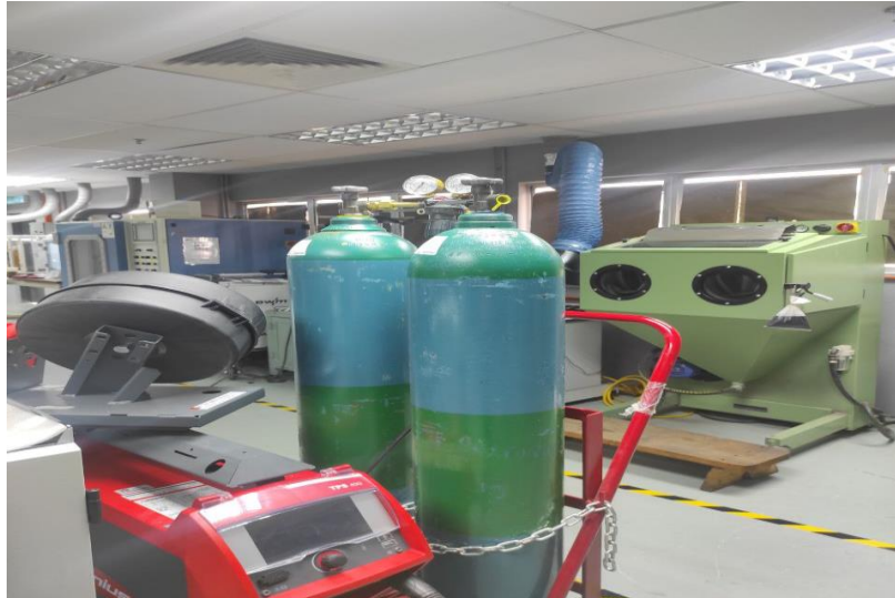
Figure 3.15 Shielding Gas (Argon + O 2 )
