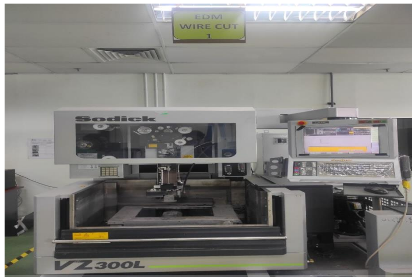
Figure 3.24 EDM Wire Cut Sodick VZ300
