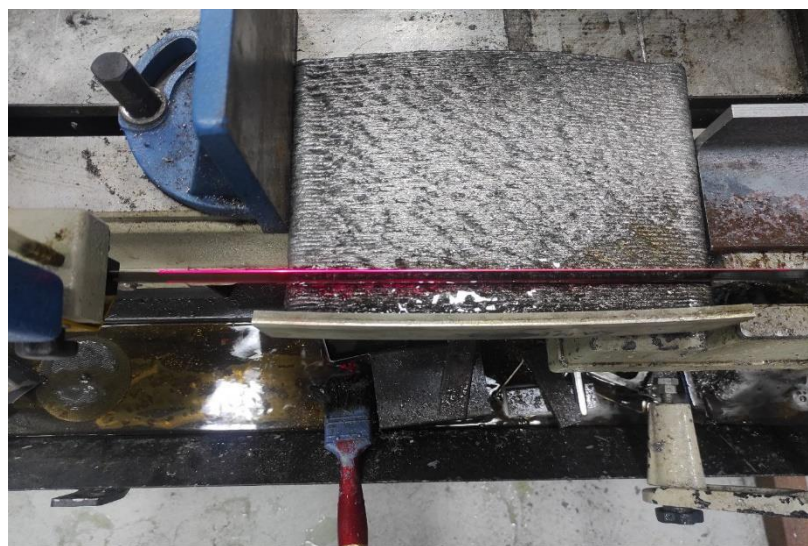
Figure 3.18 Cutting process (remove the substrate from the sample).
