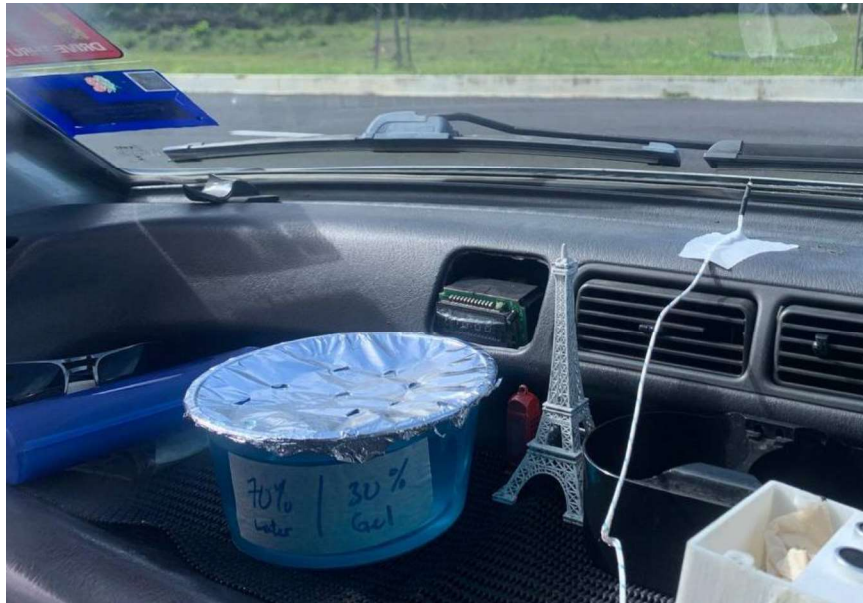
Figure 4.7 Placement of Heat Absorbent Material at Front Dashboard
