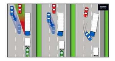
Figure 1.2 Accident Caused by Blind Spot (Kedarkar et al., 2008)
