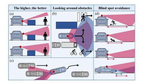
Figure 2.9 Advantages and disadvantages of different sensor mounting positions (Hartstern et al., 2020)
