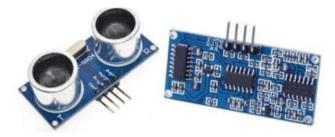
Figure 3.11 Ultrasound rangefinder HC-SR04 (Zhmud et al., 2018)
