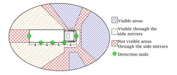
Figure 2.8 Red crossing lines indicate areas that cannot be seen through the side mirrors, or the blind spot area. The green dots are truck with all mounted detecting nodes and all surrounding blind areas, dashed and solid orange lines indicate areas that can be seen through the side mirrors, double blue lines indicate regions that can be seen through the windscreen (De Raeve et al., 2020)
