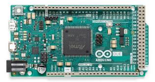
Figure 3.10 Arduino Due
