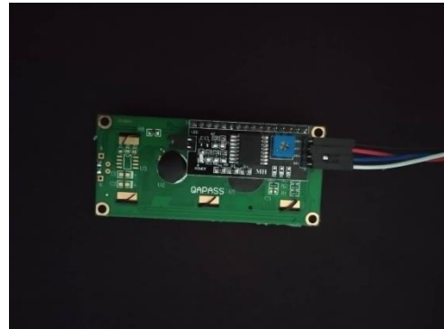
Figure 3.7 I2C Figure connect with LCD
