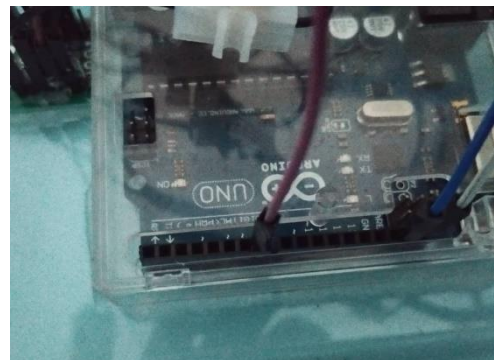
Figure 3.9 Reset wire pin and SLC with SDA wire
