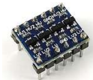
Figure 3.6.5: Logic Level Converter 4-Ch Bi-Directional Module[29]
