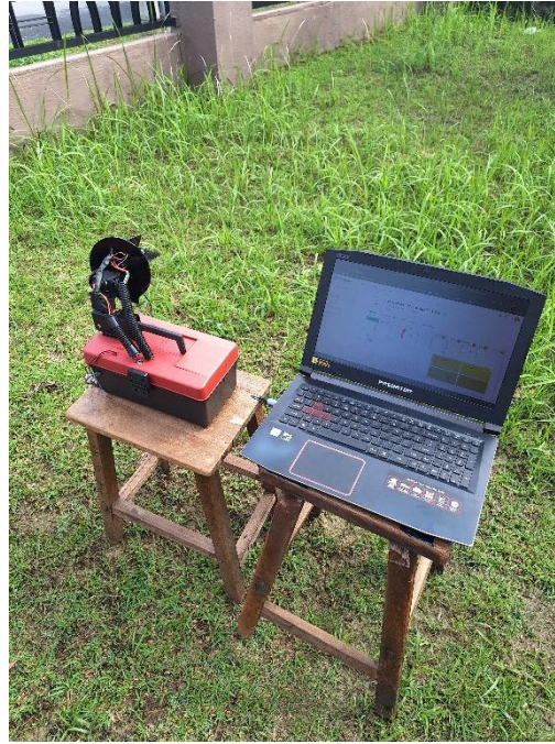
Figure 4.1 : Calibration of LDR sensors
