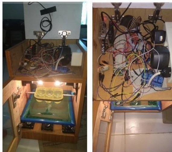
Figure 2.8 Internet of things based control and monitoring system of chicken eggs incubator using Raspberry Pi[3]
