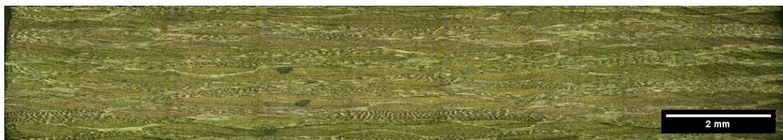
Figure 4.1: Surface of Region 2 after 0mm depth of grinding.
