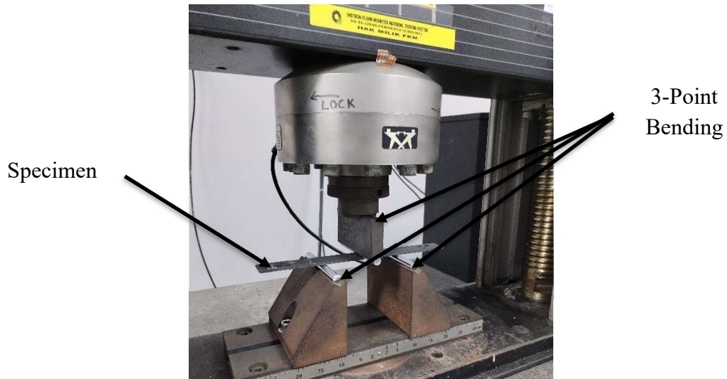
Figure 3.8: Setup of bending test using UTM.
