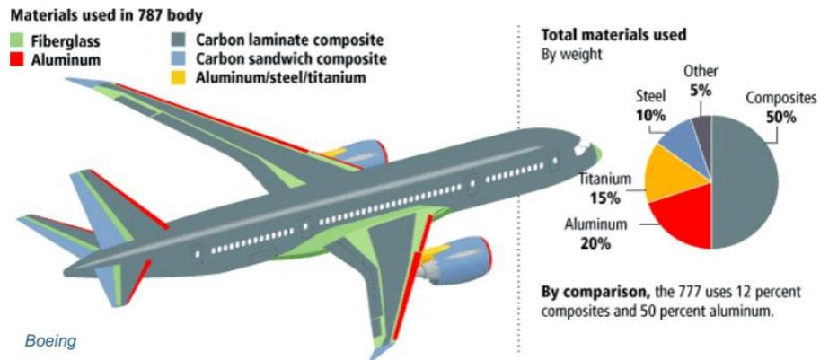
Figure 1-1: Materials used in Boeing 787 body (Aero Coating, 2014)
