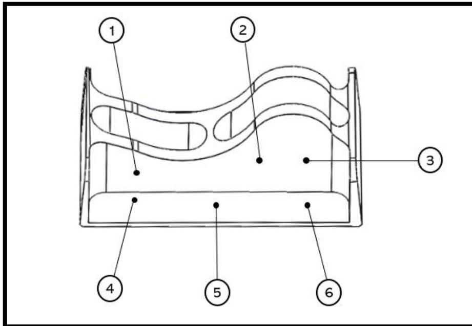
Figure 4-2: Points taken for surface roughness analysis on the right side of *open pocket*
