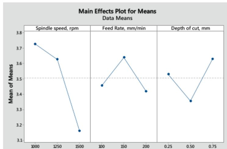
Figure 2-8: Main Effects Plot for Means of Surface Roughness (Kumar S 2020)
