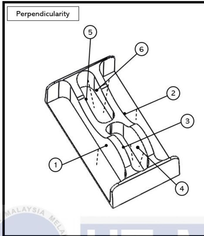
Figure 4-7: Points taken for dimensional accuracy of the *perpendicularity* aspects
