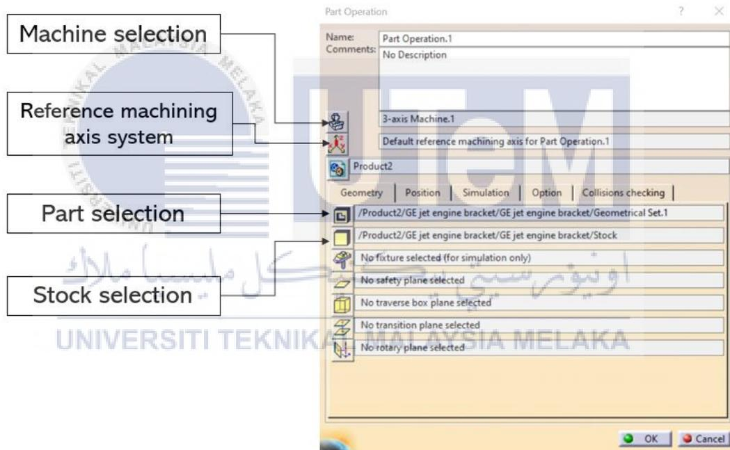
Figure 3-9: Part operation setup
