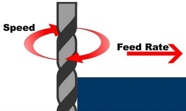
Figure 2-3: Spindle speed and feed rate movement (John, 2022)
