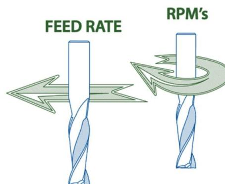
Figure 2-2: Feed rate vs spindle speed (RPM) (Woodworking Magazine, 2023)
