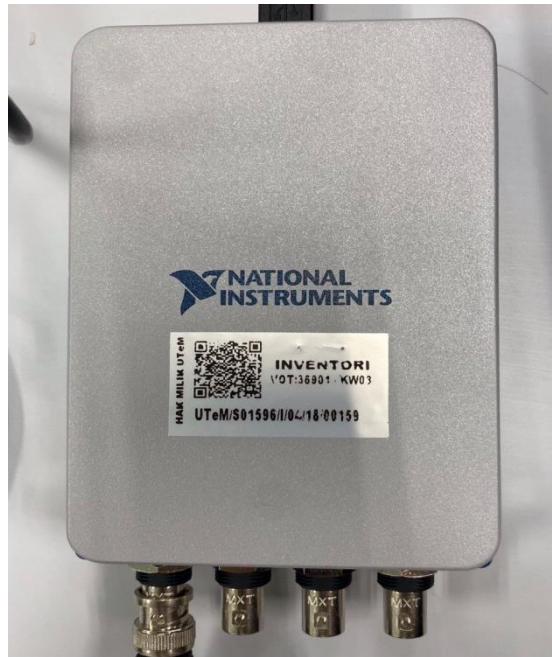
Figure 3.6 NI-9234 C Series sound and vibration input module
