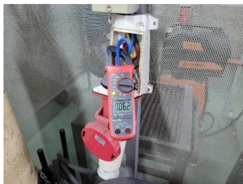
Figure 3.4 Clamping Live Wire While Experiment
