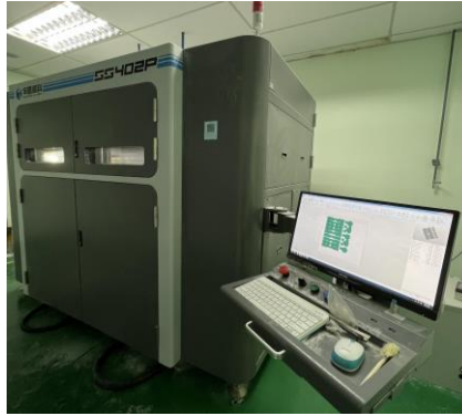
Figure 2.14: Selective laser sintering (SLS) (AMFG, 2020).
