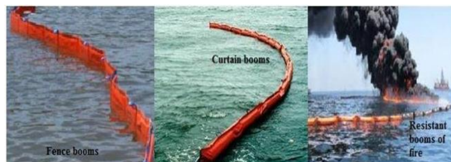
Figure 2.3: Boom types: a) Fence booms b) Curtain booms c) Resistant booms of fire (Source: Anh Tuan Hoang et al. , 2018).
